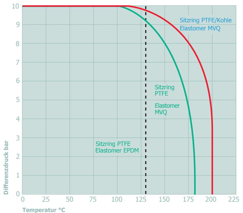
The pressure and temperature range diagram shows the application limits of the different seat ring materials.
