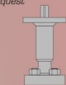
Coperchio allungato per alta temperatura Elongated cover for high temperatures
