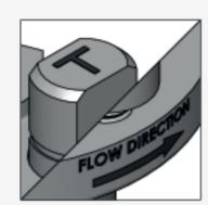
Rib and groove design between the ball and stem to guarantee the correct alignment of the upstream relief hole avoiding incorrect installations and possible malfunctions during the utilization. Once the valve is installed, the position of the upstream relief hole can be checked at any time through the top stem marking of the current position of the ball. The valve has also a flow direction identification for full integrated information.
