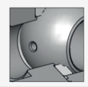
The upstream relief hole allows the relief of the excess pressure generated by a heating or a phase change ensuring the safety of the equipment
