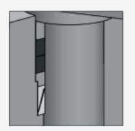
Fugitive emissions design according to ISO 15848 and TA LUFT / VDI 2440 reducing the potentially harmful emission to the environment. This design is also suitable for vacuum service up to 103 mm Hg.
